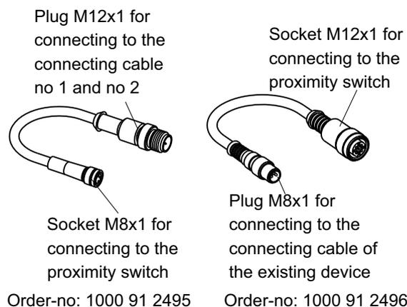
Connection cable no 1 for connection to external control units or for connection to a control with a Hirschmann plug:
