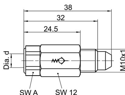
Non-return valve with plug-in connector model HP:
