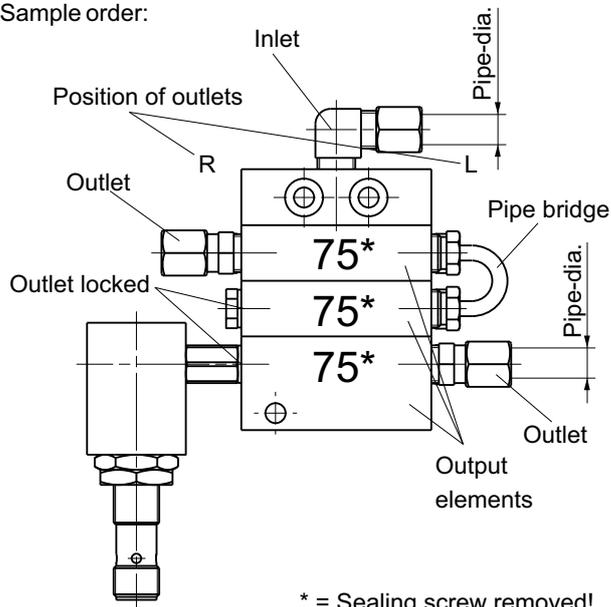
Lock screws and outlets sealed by distributor bridges are indicated by a dash (-). For distributor bridges, the sealing screw to be removed must be indicated by an asterisk (\*). Distributor disks on which a proximity switch shall be installed must be indicated with NS after the name of the dosing quantity. Proximity switches can be installed either to the left and to the right of MX-F distributors. After the note NS, the proximity switch variant must be indicated:
