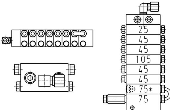
MX-F distributor 5/7, to which three distributor disks should be added:
