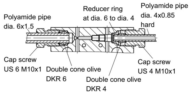
Straight pin-and-socket connector for MX-F distributor:
