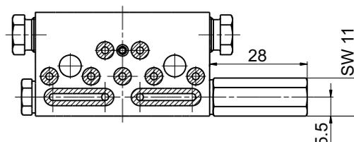
MX-F distributor with attached control pin indication (primed):
